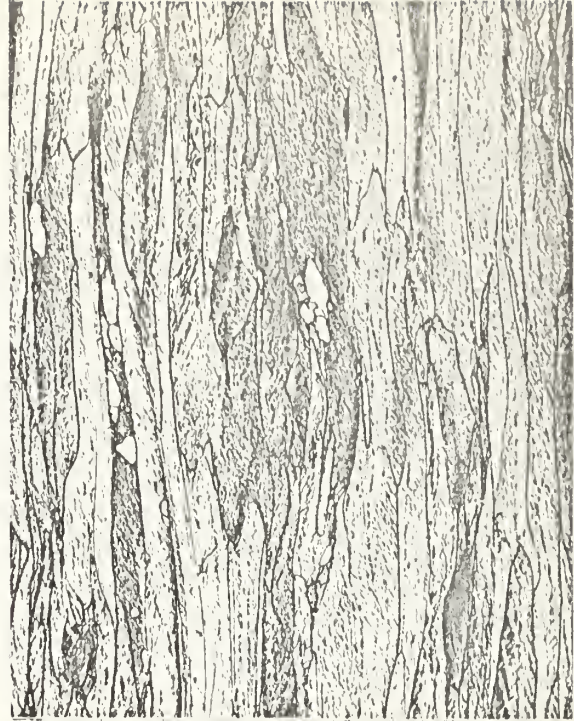
FIG. 6 AT 540°C FOR 1 MINUTE (ROCKWELL 30T 69.2)
